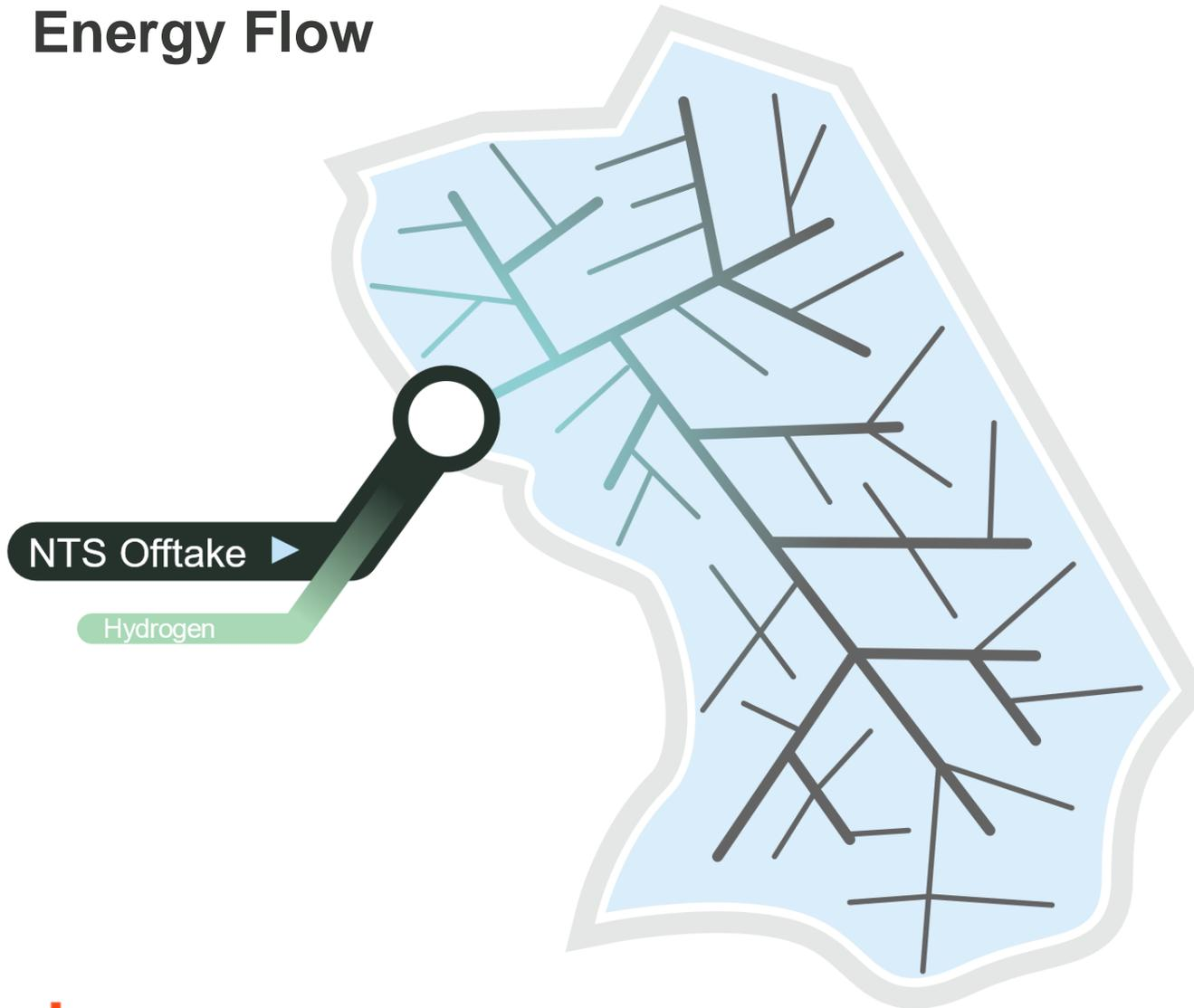
Hydrogen blend  $\leq 5\%$  at NTS/LDZ offtake C with min. CV =  $38.6 \text{ MJ/m}^3$  maintains LDZ FWACV within  $1 \text{ MJ/m}^3$  cap.
