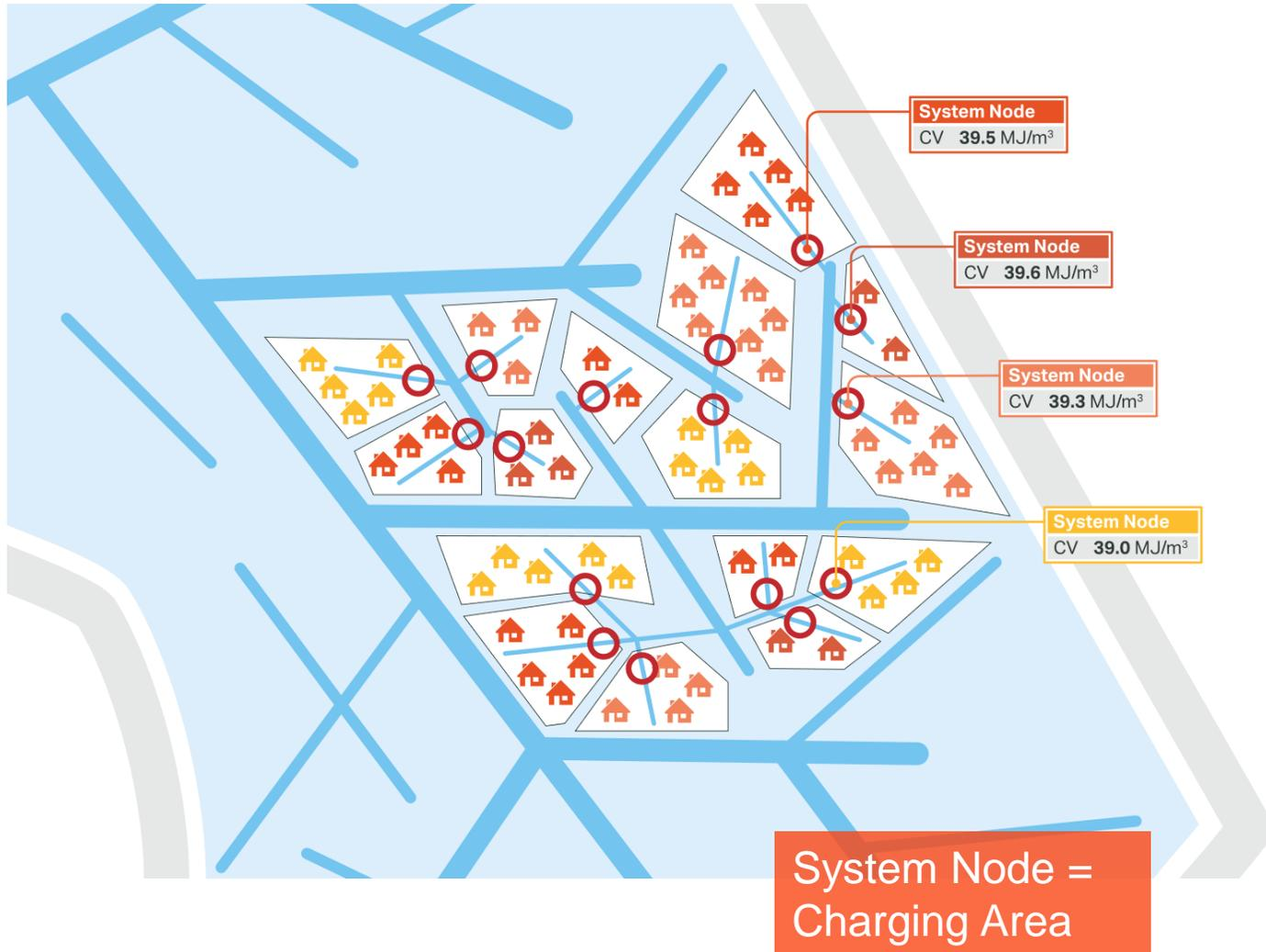
Measured CV and volumes at LDZ offtakes from NTS are inputs to online LTS model
