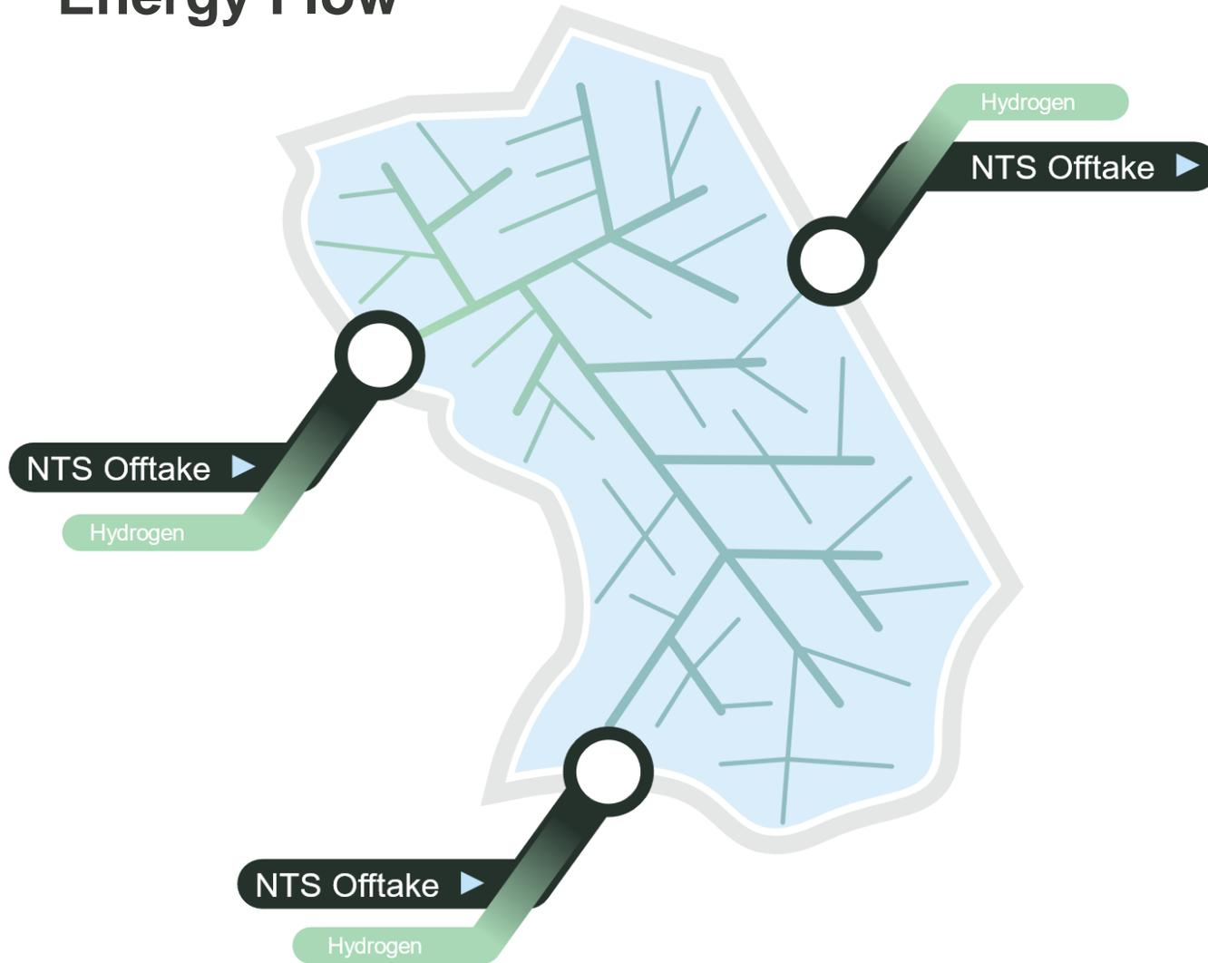
Hydrogen blend at **CV = 34 / 35 MJ/m<sup>3</sup>** from other input points supplies **>80%** of LDZ gas energy and so brings LDZ FWACV down to 35 MJ/m<sup>3</sup>, so avoiding CV cap.
