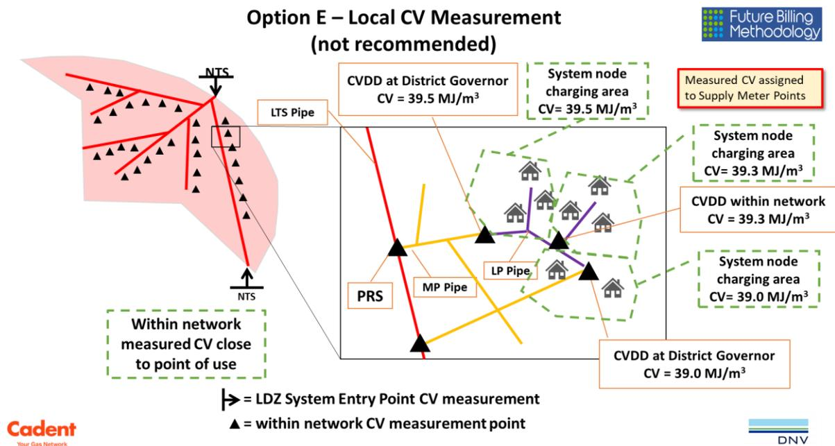
**Fig 6-6 Schematic – Option E: Local CV Measurement**
