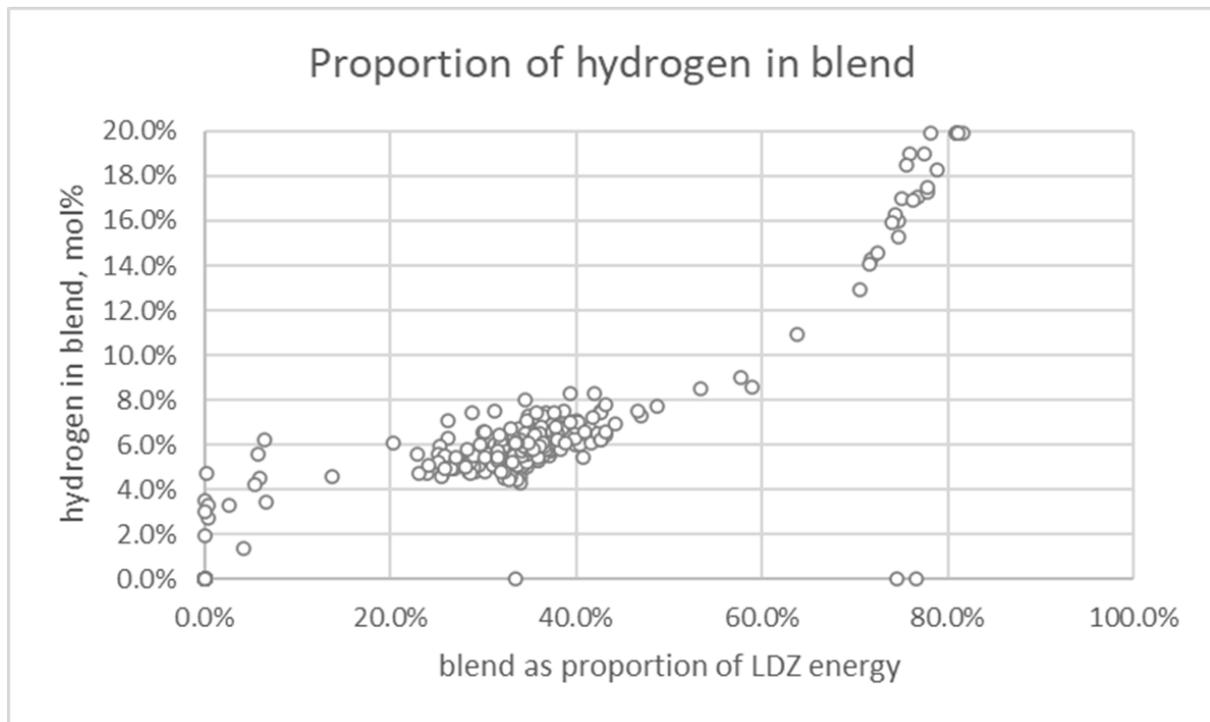
The chart above illustrates that as the proportion of LDZ energy delivered as blend (X axis) increases, this allows for a higher volumetric percentage of hydrogen (Y axis) to be blended at the injection point, as the greater proportion of lower-CV hydrogen blend acts to decrease the flow-weighted average CV across the LDZ.
