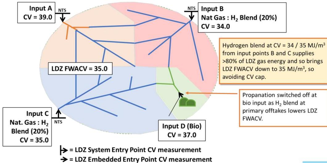
Fig. 6-2 Schematic – Option A: Blending of green gases as majority energy flow in LDZ
