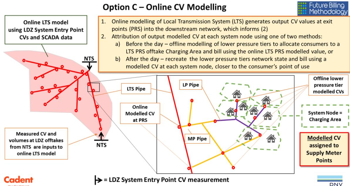
**Fig 6-4 Schematic – Option C: Online CV Modelling**
