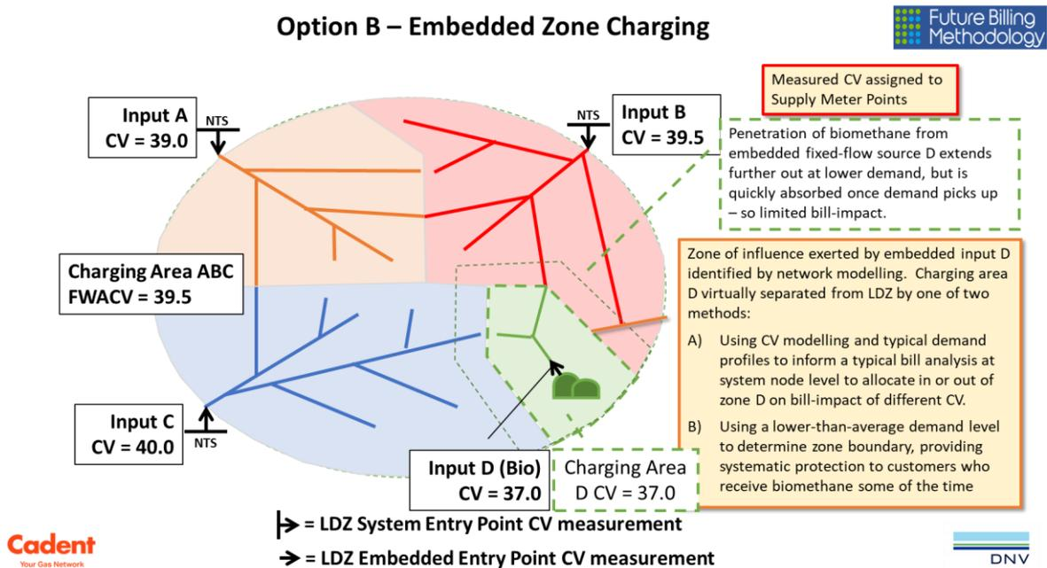
Fig. 6-3 Schematic – Option B: Embedded Zone Charging
