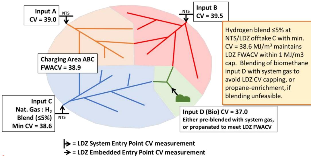
Fig. 6-1 Schematic – Option A: Blending of green gases as minority energy flow in LDZ
