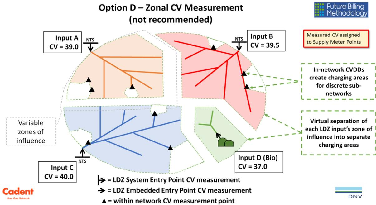
**Fig 6-5 Schematic – Option D: Zonal CV Measurement**
