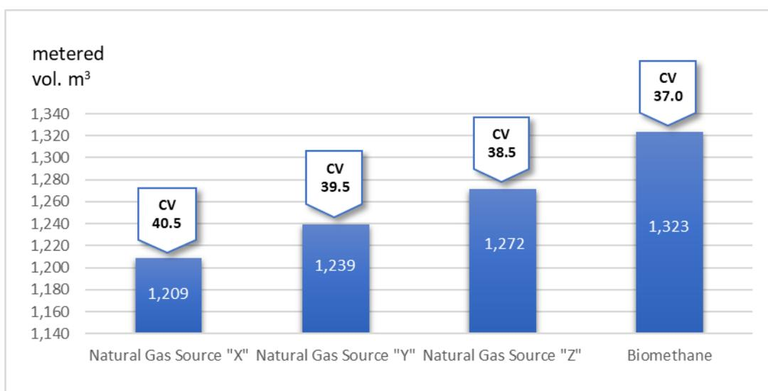
The chart above illustrates how gases of progressively lower CV require a greater volume through the consumer’s meter to meet the same fixed energy requirement. The CV of each gas (stated in megajoules per cubic metre or MJ/m<sup>3</sup>) is shown above each column. At 37 MJ/m<sup>3</sup>, un-enriched biomethane would require around 9.5 per cent more volume to deliver the same heat output as natural gas source “X”, at 40.5 MJ/m<sup>3</sup>.
